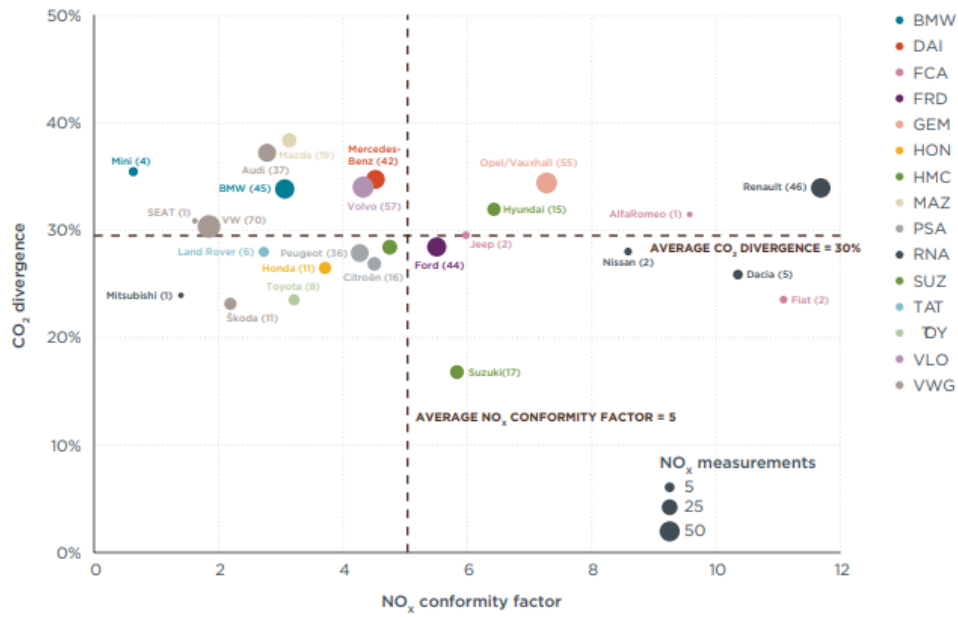
Figure ES-3: Euro 6 diesel passenger car gap between real-world and type-approval CO 2 emission values vs. on-road NO x emissions conformity factors by manufacturer. 4
